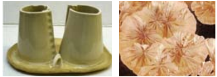
Fig. 4. Zinc oxide calcined (left) and raw (right) in close up of a crystalline glaze (contains 25 % zinc) with high expansion (low crazing) body [9-10].
