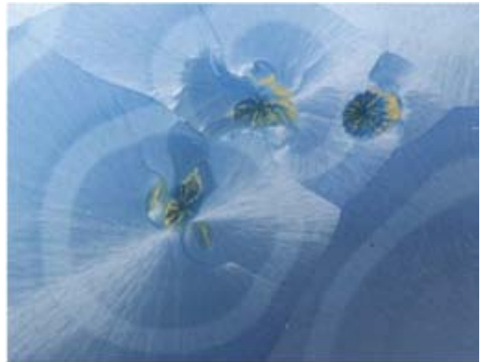
Fig. 19. Spherulitic crystallization in a glass [65].
