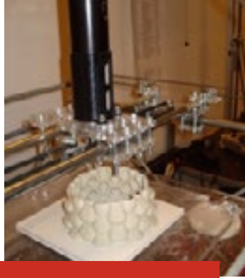
Görsel 3.4. Kartezyen tipi yazıcı, Unfold, Antwerp Foto: yazar Figure 3.4. Cartesian type printer, Unfold, Antwerp Photograph: Author
