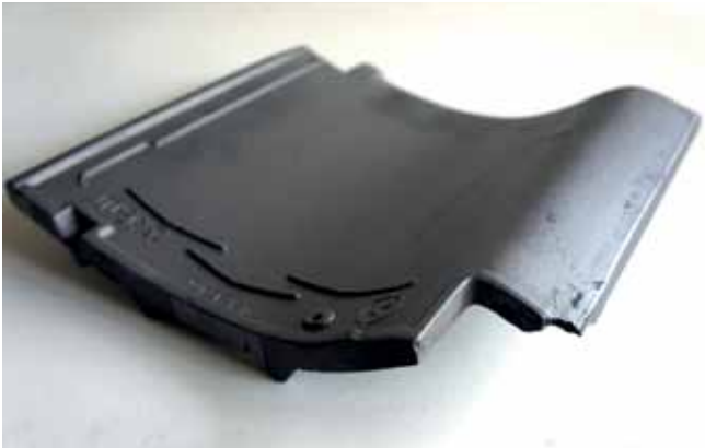
Kusurlu kiremit, kusursuz malzeme Faulty tile, faultless material
