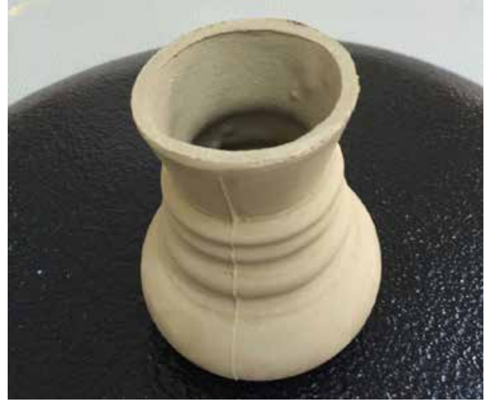
(c) Figure 3: Slip cast form of Kastamonu Mud containing (a) 20 wt% (KM20) (b) 30 wt% (KM30) clays (c) KM20 after sintering at 1150°C .
