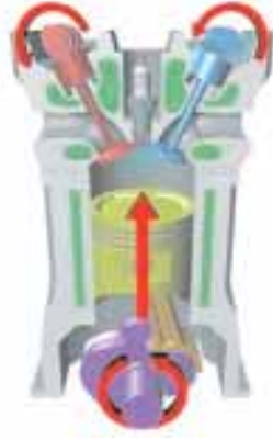
Şekil 1: İçten Yanmalı Motorun Kesiti 1 Figure 1: Cross-Section of Internal Combustion Engine 1
